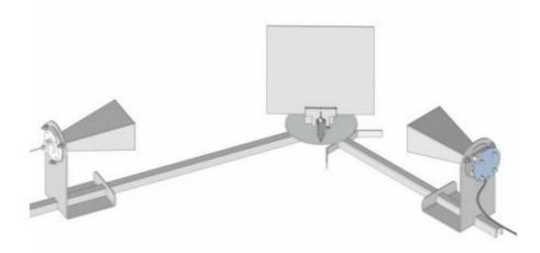
Set up the reflector plate at an angle of  $30^{\circ}$  using the indicators on the base. Adjust the receiver so that the received signal is at its maximum and measure this angle on the base. Repeat this with,  $40^{\circ}$ ,  $50^{\circ}$  and  $60^{\circ}$ . What can you conclude about the relationship between the angle of reflection and the angle of incidence for electromagnetic waves? Explain all observations in your lab report.
